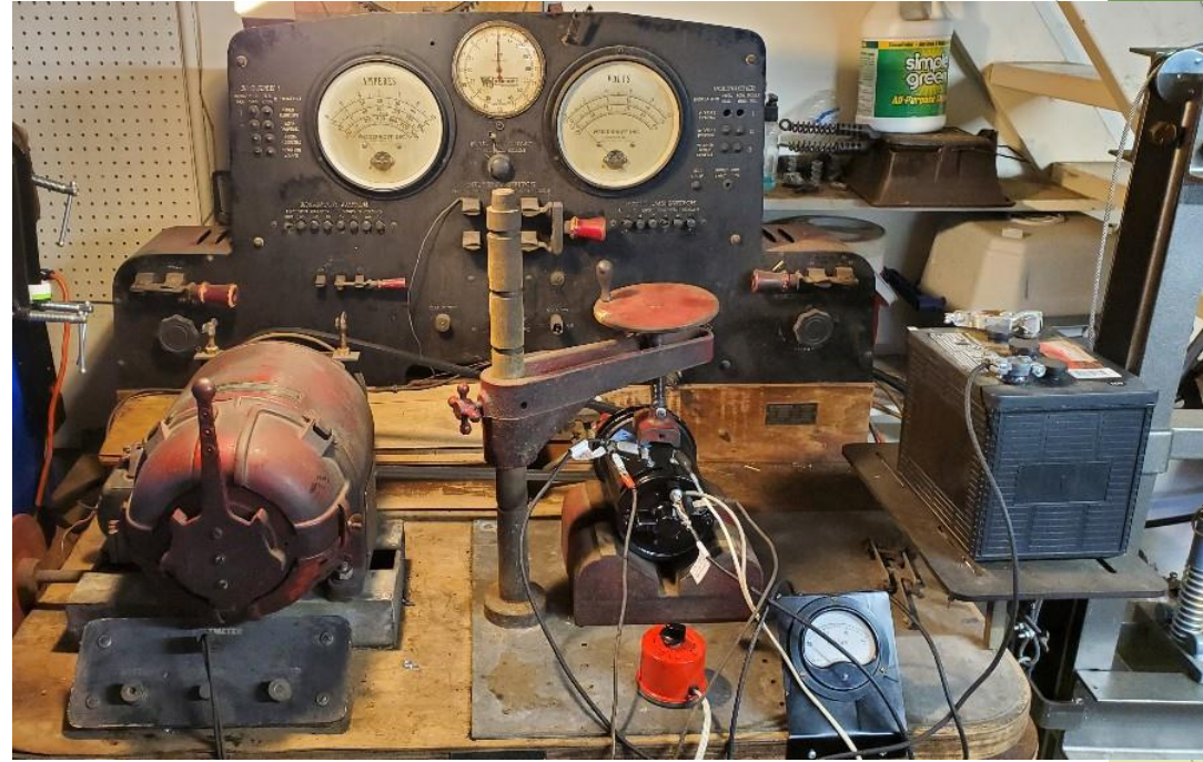
Early 1930s Weidenhoff Generator Test Bench
